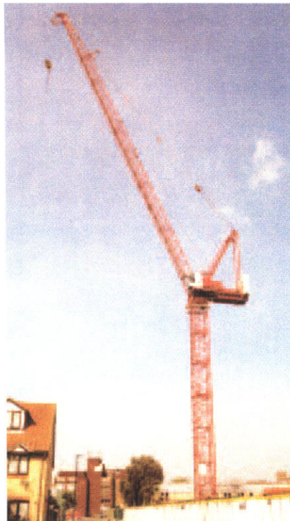
For a house building site at Luking Street, Kier Plant delivered this Liebherr 160 HC-L with 55 m jib. In the one fall operation 8 tonnes can be lifted to 25 m radius and 2 tonnes at 55 m radius
