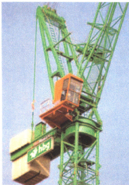
At the 55 Baker Street project this Wolff 180B, the best selling Wolff luffing jib model, is working in the colours of HBG, rented from HTC, alongside two Wolff 100Bs and one 6522FL-6. The 58.5 m free standing 180B is rigged with 55 m jib for a 2.5 t tip load
